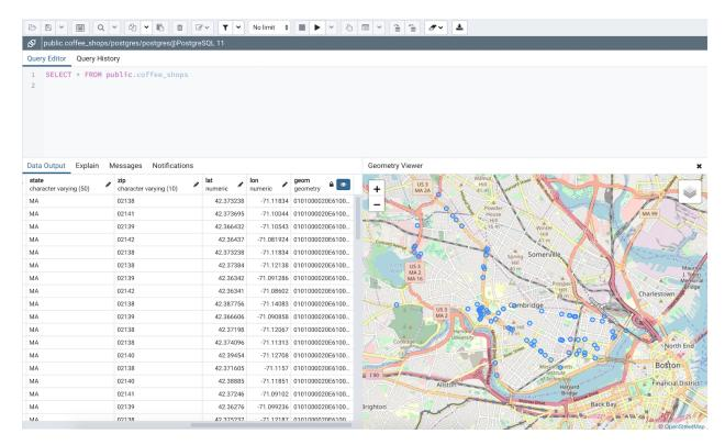
You can adjust the layout by dragging the title of the panel. To view the properties of the geometries directly in map, just click the specific geometry:
