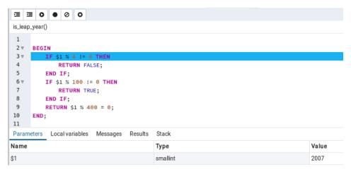
The lower panel of the debugger window provides a set of tabs that allow you to review information about the program:
